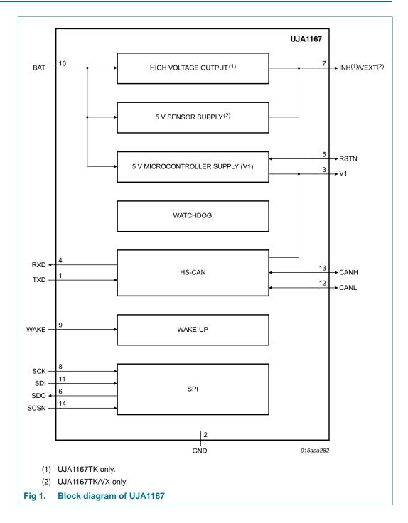
Mini high-speed CAN system basis chip with Standby/Sleep modes & watchdog
