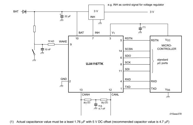
(2) For bus line end nodes,  $R_T = 60 \Omega$  in order to support the 'split termination concept'. For sub-nodes, an optional 'weak' termination of e.g.  $R_T = 1.3 k\Omega$  can be used, if required by the OEM.
