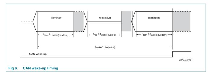
When a valid CAN wake-up pattern is detected on the bus, wake-up bit CW in the Transceiver event status register is set (see <u>Table 22</u>) and pin RXD is driven LOW. If the SBC was in Sleep mode when the wake-up pattern was detected, V1 is enabled to supply the microcontroller and the SBC switches to Standby mode via Reset mode.
