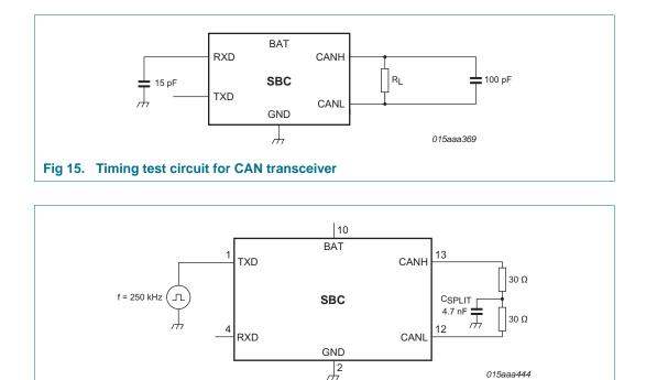
Fig 16. Test circuit for measuring transceiver driver symmetry
