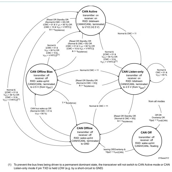
Fig 5. CAN transceiver state machine (with FNMC = 0)
