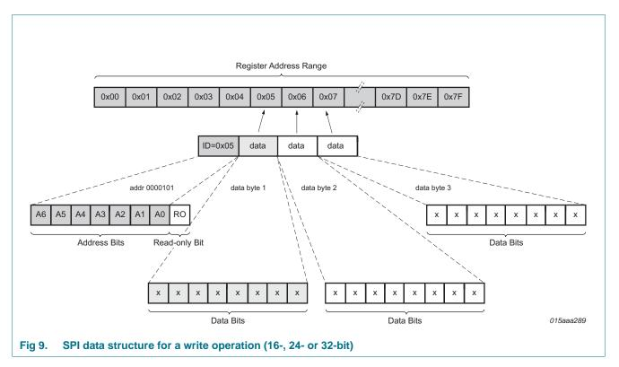
During an SPI data read or write operation, the contents of the addressed register(s) is returned via pin SDO.
